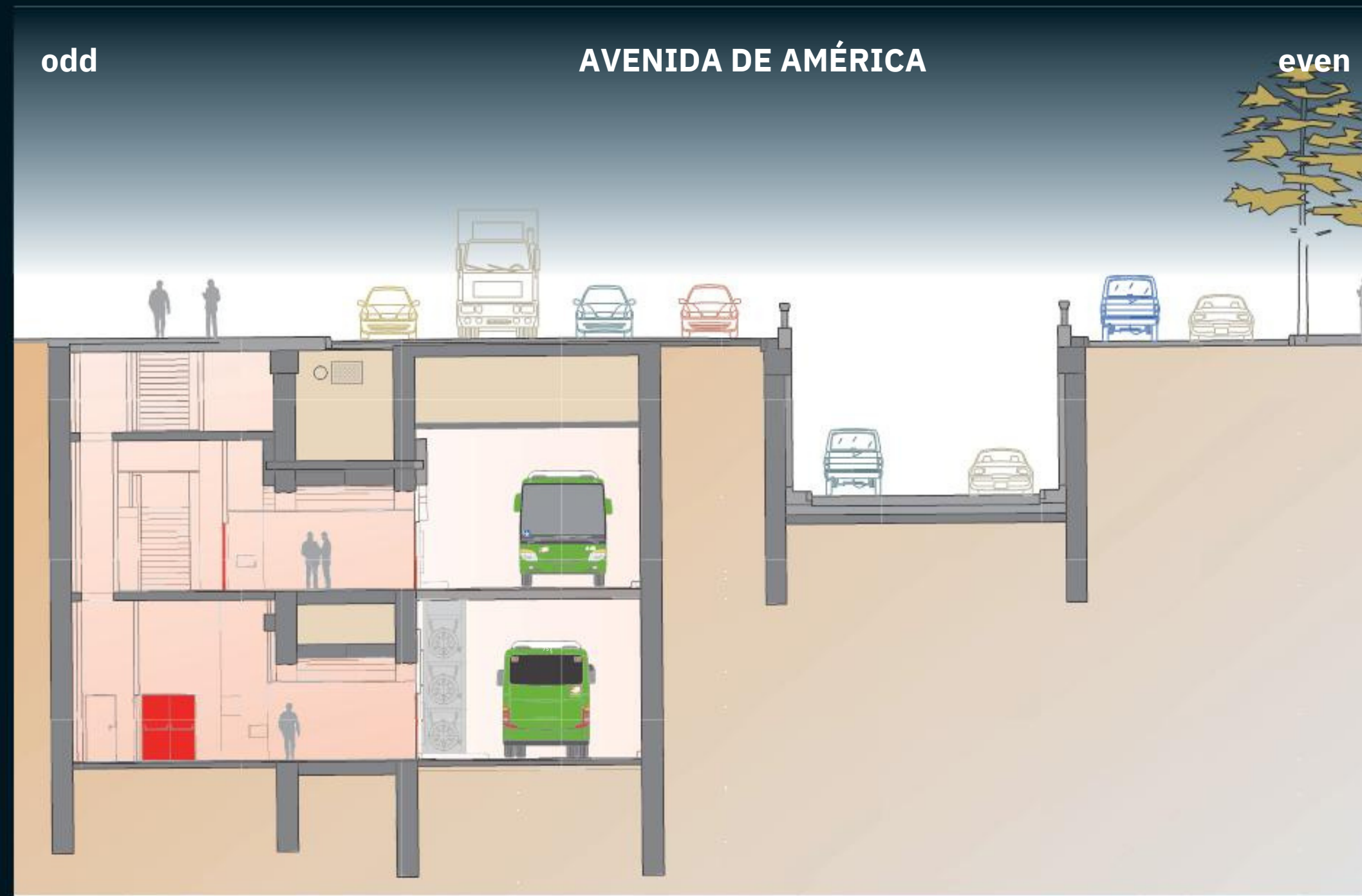
Double-height tunnel section
